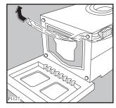
Remove the polystyrene base. Set the machine upright and unscrew the remaining rear screw. Slide out the relevant pin.
